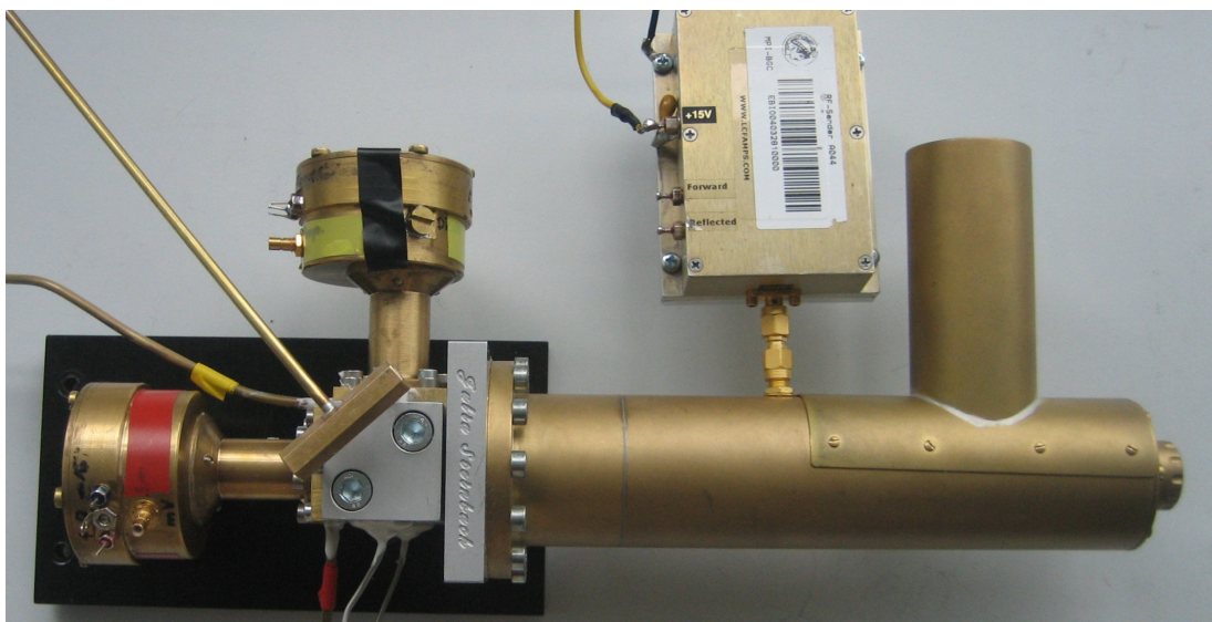
Figure 4.6: Design of ICON's main part, including sample cells, beamsplitter, phototube detectors, amplifying electronics, xenon lamp and RF power supply
