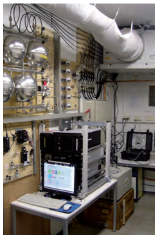
At ZOTTO, the spherical buffer volumes (top left) allow a near-concurrent measurement of air from all six inlet heights with a single analyser.
