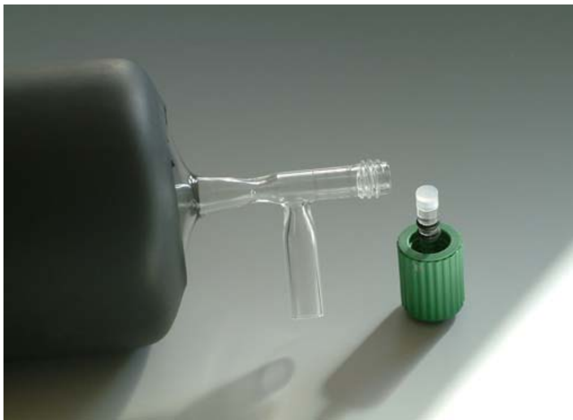
Figure 2; Glass flask with PCTFE-on-glass seat 4 . The shaft seal is made using two Viton O-rings. The flasks are protected against ex- or implosion hazards by a heat shrink hose (black).
