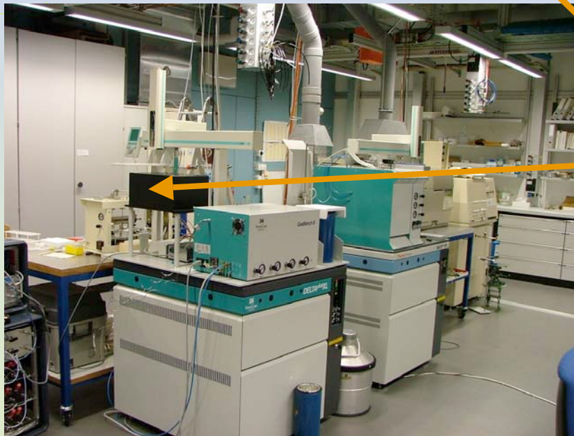
In the lab: Determination of Stable C and O isotope ratios with an IR mass spectrometer
