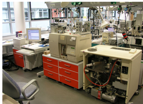
Simon (Delta C; 'Stable Isotope Monitoring System') Delta C prototype IRMS (Finnigan MAT); the instrument is coupled on line with an EA 1100 (CE, Maastricht) via a ConFlo III interface
