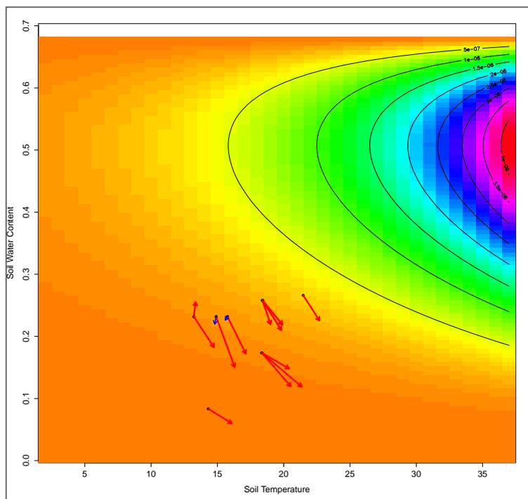
*Sensitivity of soil organic matter decomposition to simultaneous changes in temperature and moisture. Points represent the combination of soil temperature and soil water content of the control treatment of experiments, and arrows represent the direction of change imposed by the treatments. Red arrows represent soil warming while blue arrows cooling. Contours and colors in the background represent model predictions of the sensitivity of reaction velocities for enzymes.*
