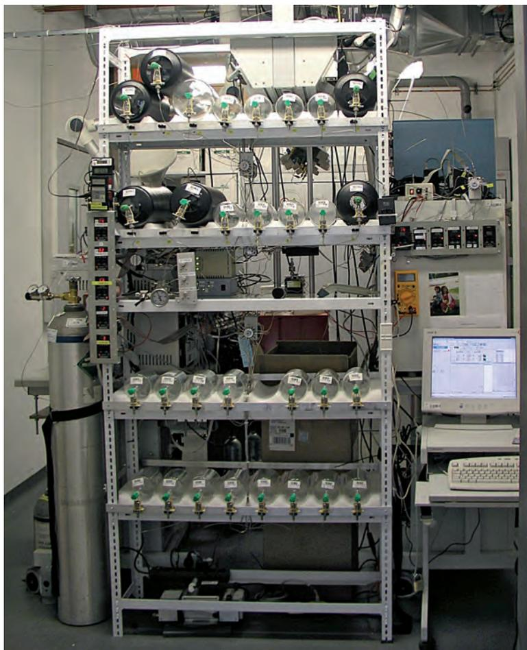
*Gas chromatographic system for trace gas analysis of air samples*
