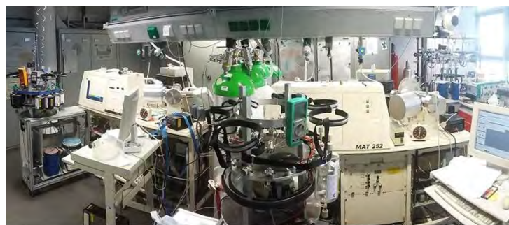
Two MAT 252 (Thermo Finnigan) isotope ratio mass spectrometers (IRMS) coupled to homemade BGC-Air Traps, that separate CO 2 from the other air components. These two systems are used for δ 13 C and δ 18 O analyses of CO 2 in air, and the production of JRAS-06 CO 2 -in-air reference standards. Photo: H. Moossen
