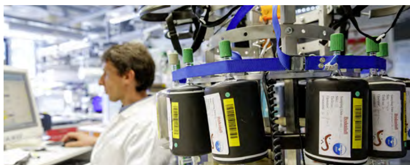
Flask autosampler on the BGC-Air trap. Here atmospheric samples from sampling stations situated all over the world are analysed. Photo: A. Schroll
