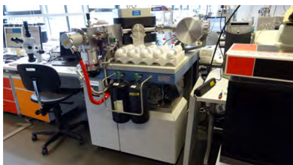
Dual inlet sector field mass spectrometer (MAT 253) for high-precision analyses of pure \text{CO}_2 gas. Photo: S. Héjja
