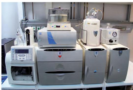
Ion chromatography system with amperometric detector, 'ICS-3000' from Dionex
