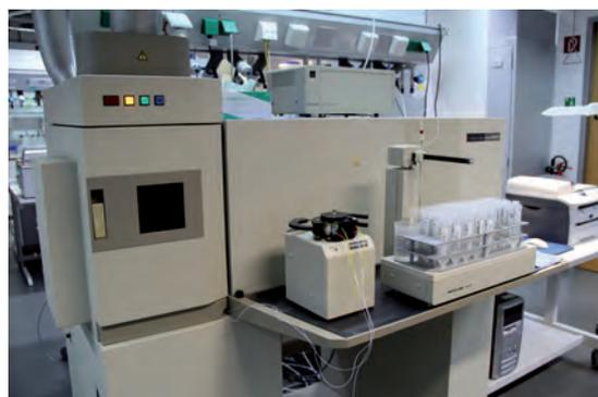
Atomic emission spectrometer with inductive coupled plasma (ICP), 'Optima 3300DV' from Perkin Elmer
